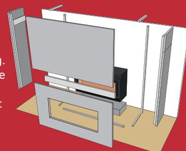
Most enclosures can be built using only SKAMOTEC 225, replacing the need for light-frame construction and wall covering. This eliminates a complete stage in the construction process, combining multiple building materials into one.
